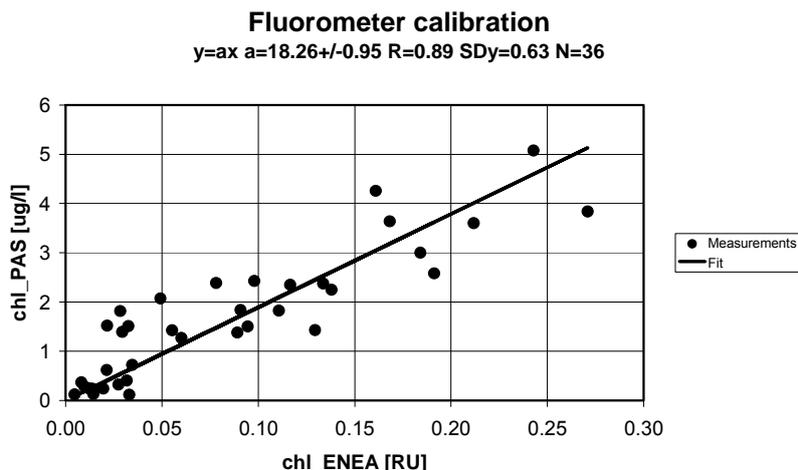
Figure 4: Intercomparison between spectrometer ( $\mu\text{g/l}$ ) and spectrofluorometer data (RU).
