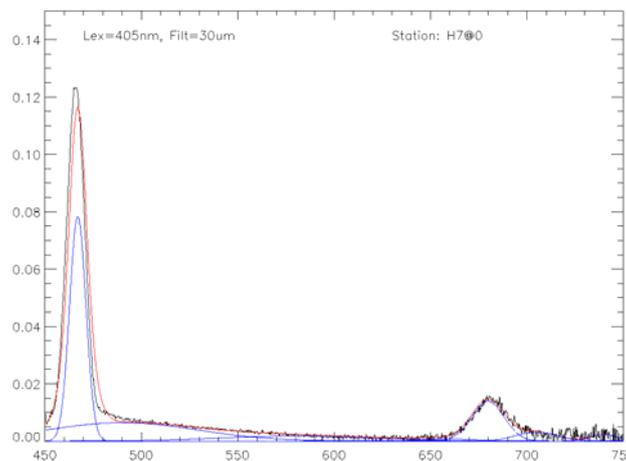
Figure 3: Fitting procedure of measured fluorescence spectrum (black line), Gaussian functions (blue lines) and final fitted function (red line) ( $\lambda_{exc} = 405 \text{ nm}$ , filtration: 30  $\mu\text{m}$ . Sample H7, superficial).
