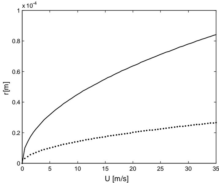
Fig. 1. Turbulent diffusion dominated particle sizes as a function of wind speed. Solid line  $r = (9\rho_p\nu U_*/2\rho_w g)^{1/2}$ ; dotted line  $r = 0.1(9\rho_p\nu U_*/2\rho_w g)^{1/2}$ .
