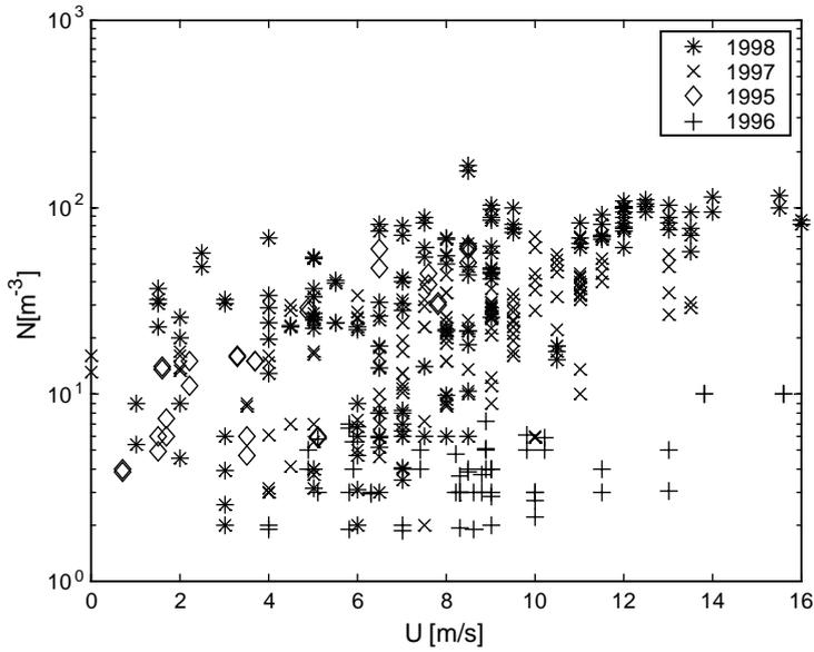
Fig. 5. Particle concentration versus wind speed (for size range 4.5–5.5  $\mu\text{m}$ , Arctic Seas).
