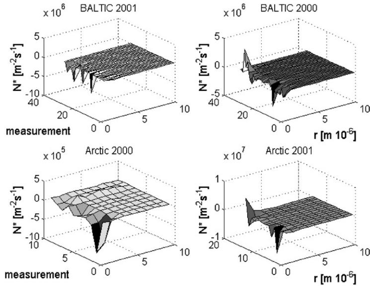
Fig. 3. Scale  $N_*$  of aerosol concentration. Each graph represents result from one cruise. The vertical axis on all 4 graphs represents  $N_*$  scale value, as a function of particle radius for the all measurements in single cruise (left horizontal axis is the sequential number of the measurement).
