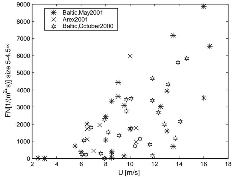
Fig. 4. Number particle flux versus wind speed (for size range 4.5–5.5  $\mu\text{m}$ , Arctic Seas and Baltic Sea).
