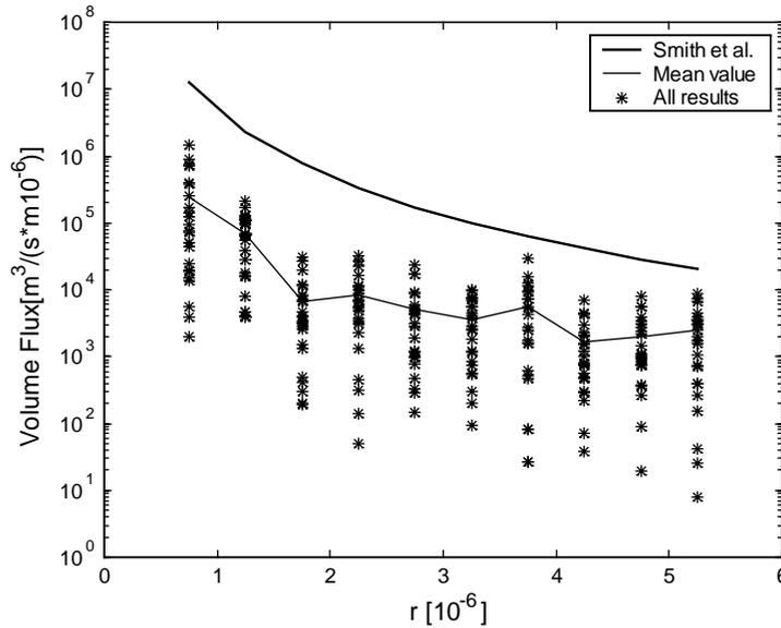
Fig. 9. Sea spray generation function as a volume flux, that is, as  $4\pi r^3/3 dF/dr$ .
