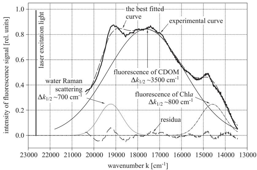
**Fig. 2.** Typical lidar-induced seawater fluorescence signal
